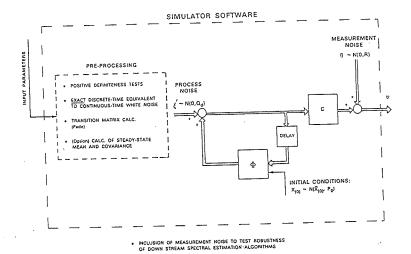
Figure 2. State-variable Markov-based Monte-Carlo simulator.
