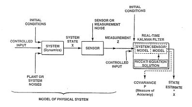
Figure 1. Overview functional block diagram of the internal structure of a Kalman filter.
